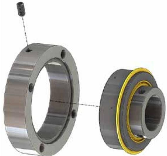
8. Reverse the process and apply thread locking fluid (loctite) to the set screws
