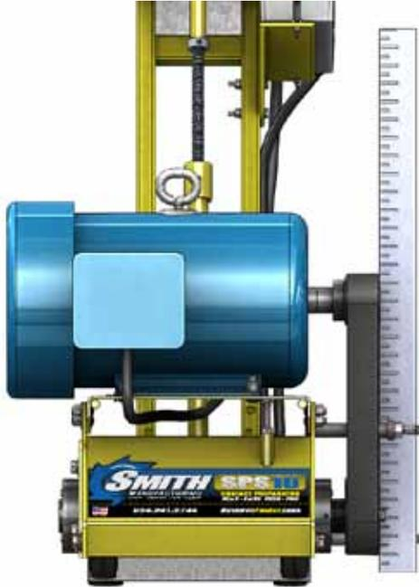
16. Now tighten the rear securing bolts with the two 9/16" wrenches.
