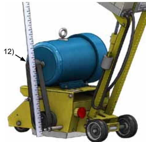
13. After installation, use the 3/8" open-wrench to screw out the belt tensioning jackscrew under the motor plate to tension the belts to your desired tension. Do not over-tension the belt.
