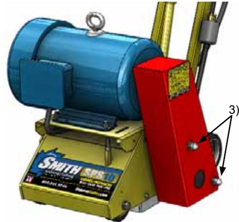
5. Lubricate the motor plate (belt tensioning) jackscrew with WD40 on the front left of the machine.
